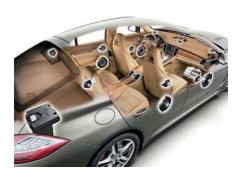
The new Porsche Panamera from the Stuttgart-based manufacturer comes with the option of installing a first-rate high-end surround sound system which was developed in close cooperation with the manufacturer Burmester from Berlin. The high-end surround sound system consists of 16 separate amplifier channels with more than 1000 watts of overall power, and a prodigious
