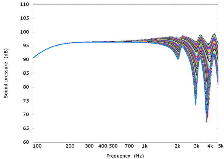
Figure 1.7. Simple cone loudspeaker 1m polar response at 2 degree angular increments.
