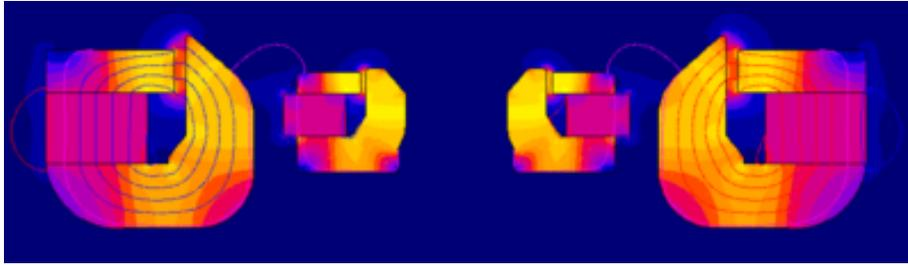
*Figure 1.15. Computer analysis of Uni-Q magnet system*
