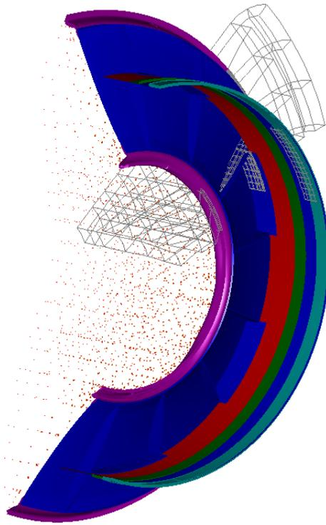
Figure 1.13. Rear sectional view of the Concept Blade midrange cone, taken from a computer model.
