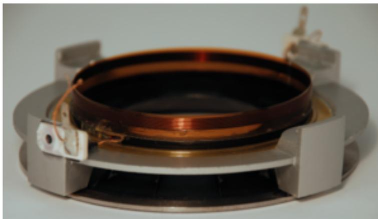
*Figure 1.16. Rear view of midrange front assembly showing voice coil.*
