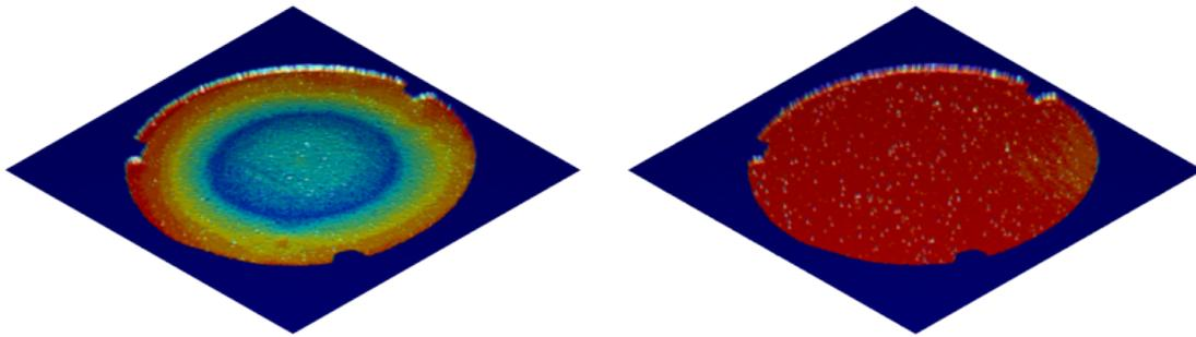
Figure 1.2. Laser vibrometer scan of tweeter dome in breakup (left) and piston-like (right).
