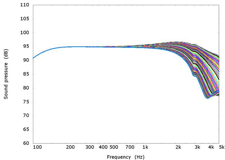
*Figure 1.12. Ribbed cone loudspeaker driven at node of first resonance, 1m polar response at 2 degree angular increments.*
