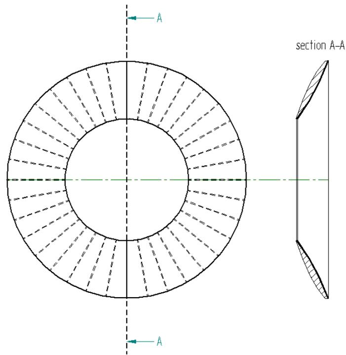
Figure 1.10. Loudspeaker cone with reinforcing ribs.
