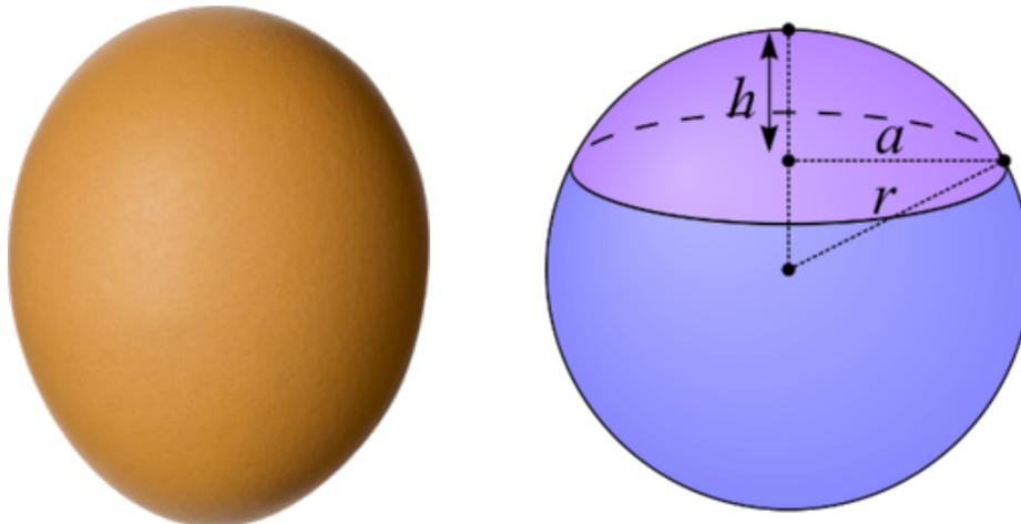
Figure 1.3. The rounded end of an egg (left) is close to the best dome shape mechanically but a spherical cap is the optimum for acoustical performance (right).
