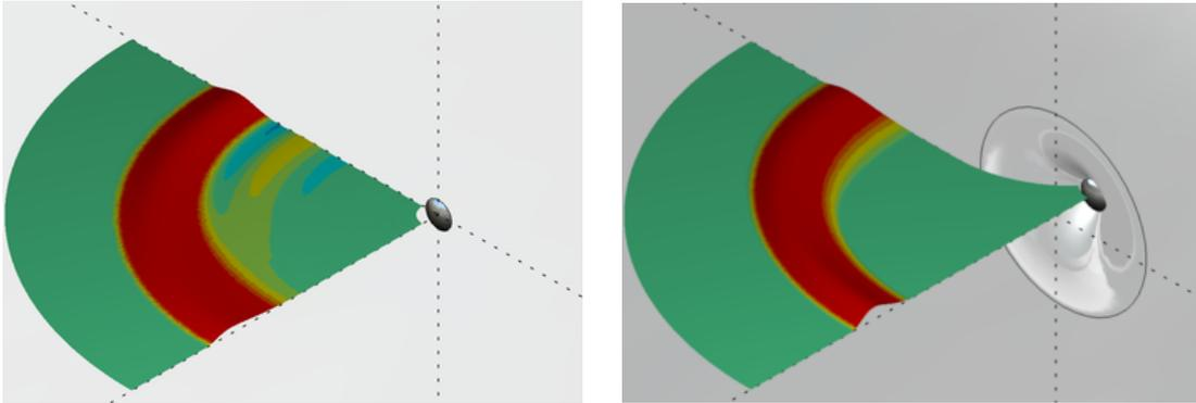
*Figure 1.1. Conventional tweeter in a baffle (left). Uni-Q tweeter in a baffle (right).*
