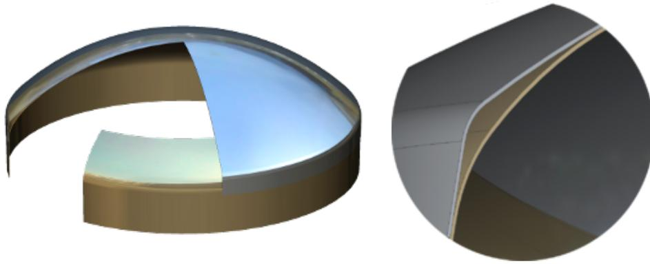
*Figure 1.4. The Concept Blade uses a Stiffened Dome from two parts which form a triangular strut massively increasing the rigidity of the dome.*
