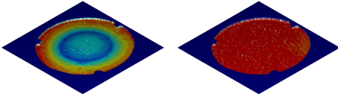
Figure 1.2. Laser vibrometer scan of tweeter dome in breakup (left) and pistonic (right).
