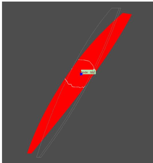
Figure 1.11. FEA Modal analysis to determine the nodal position of the ribbed cone at first resonant frequency.
