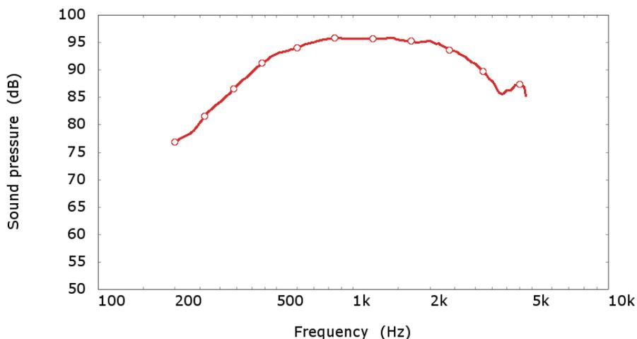
Figure 1.14. In cabinet measurement of midrange driver frequency response.
