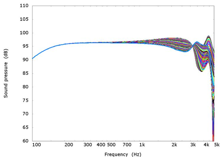
Figure 1.9. Cone loudspeaker driven at node of first resonance, 1m polar response at 2 degree angular increments.
