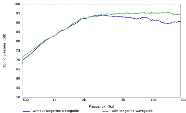
Figure 1.6. Concept Blade tweeter response with (green) and without (blue) tangerine waveguide fitted.
