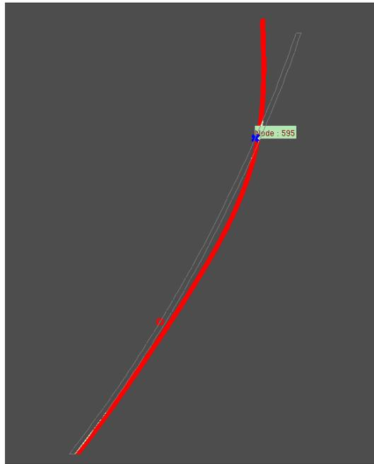
Figure 1.8. FEA Modal analysis to determine the nodal position of the cone at first resonant frequency.
